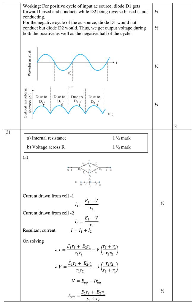
$$r_{eg} = \frac{r_{1}r_{2}}{r_{2} + r_{1}}$$
