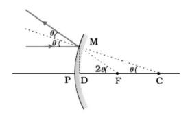
Let C be the centre of curvature of mirror, MD be the perpendicular from M to the principal axis.
